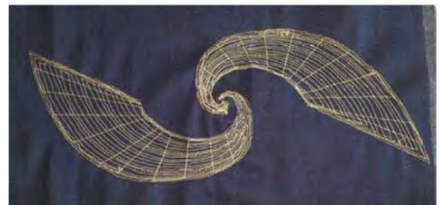
Fig. 5. Embroidered textile spiral logarithmic antenna [62].
